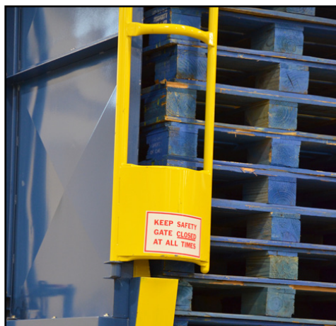
> Swinging gate for operator safety
