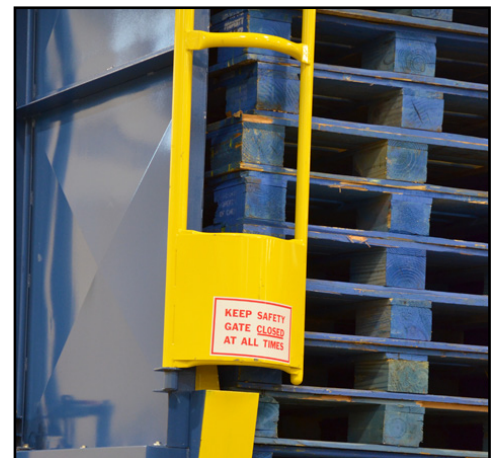
> Swinging gate for operator safety
