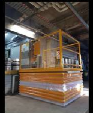
Cronulla RSL Club – Pit Mounted Dock Lifter
